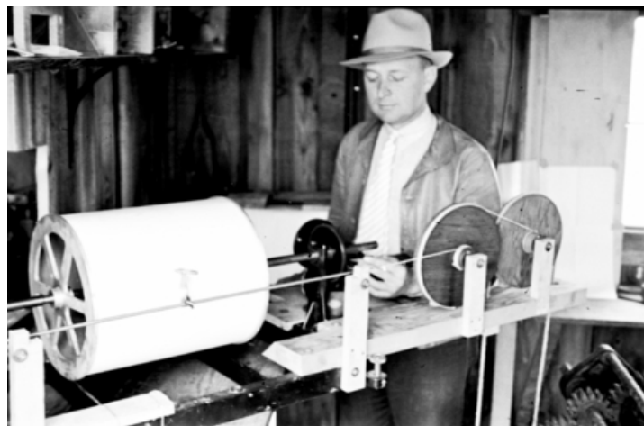
Figure 2: “Eugene Cecil LaFond [circa 1938] standing by his wave recorder installed near the end of the Scripps pier.” Eugene LaFond Papers, 1937-1939, BOX 18, FOLDER 16, Scripps Institution of Oceanography Archives.
